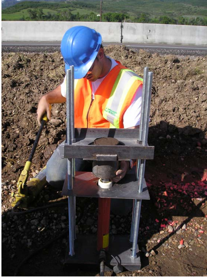
FIGURE 3.10 Extruding cement-treated specimens.
