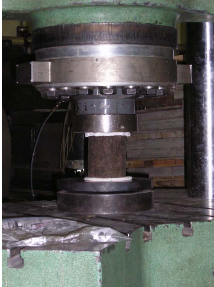
FIGURE 3.16 Unconfined compressive strength testing.
