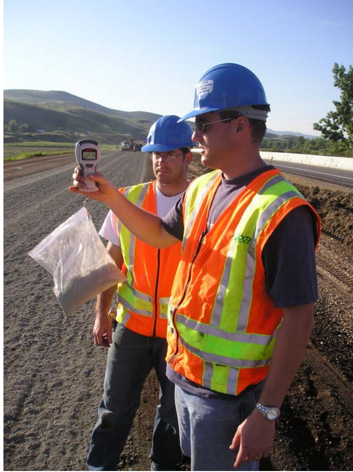
FIGURE 3.7 Measuring weight of retrieved cement.
