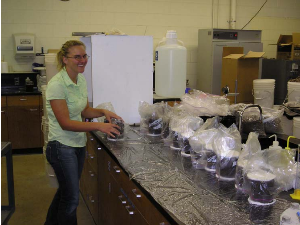
FIGURE 3.15 Preparing gypsum caps for UCS testing.
