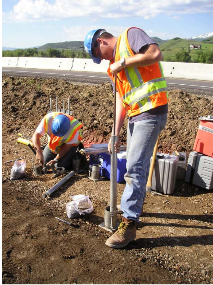
FIGURE 3.9 Compacting cement-treated specimens.
